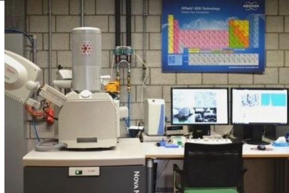
Picture of FEIs Scanning Electron Microscope at the university of Pforzheim. The EDX detector is adapted from the left side to the chamber
